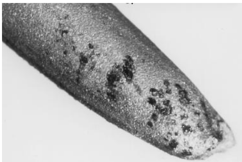
Fig.2 Multiple spots on the tip of a tin wire. Viewing under a low-power microscope reveals the rough surface of the wire (magnification 22 ×)
